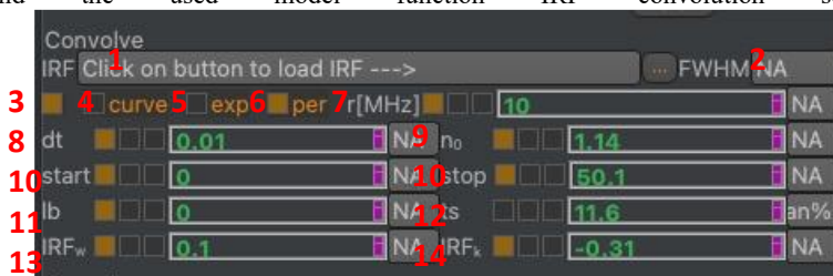
Fig.20). Certain convolution settings could be optimized during fitting or varied during sampling. However, usually, the convolution parameters are fixed. Nevertheless, convolution settings can be treated as a variable model parameter.
