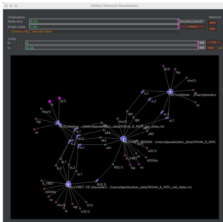
Fig.36. User interface of the Global view plugin. The plugin represents models and parameters in graphs (bottom). The Visualization group box of the plugin gathers options controlling the graph visualization (Node size, Graph scale). The Network group box can be used to save and load dependencies. The Link group box can be used to introduce and delete (clear) dependencies across selected and all parameters.
