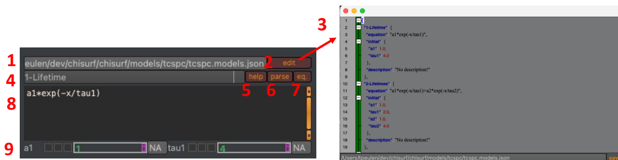
Fig.23 Fluorescence decay equation parsing. (1) A JSON file with a set of pre-defined equations for time-resolved fluorescence is shipped with ChiSurf. (2) The edit button opens a (3) JSON file editor that can be used to edit the pre-defined equations. (4) A dropdown menu lists the pre-defined equations. (5) Descriptions/help on the pre-defined equations can be enabled/disabled. (6) Parse button to update the model when equation was edited. (7) Button to enables/disables displaying the an editing equations. (8) equation editor. (9) Representation of parameters extracted from equation.
